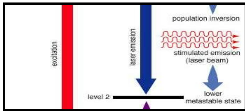
Figure (1.2): Shows the three-level laser [4].
