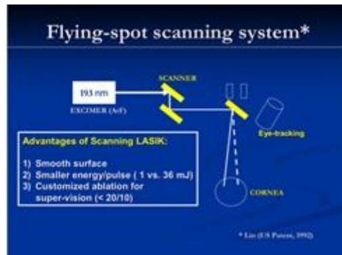
Figure (2.10): Shows a scanning Lasik system using a small flying spot for customized vision corrections (JT Lin, US patent, 1993) [27].
