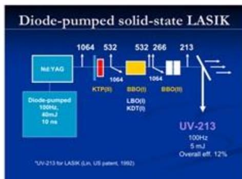
Figure (2.9): shows a patented system using a solid-state (213 nm) laser for PRK and LASIK (JT Lin, US 1992 patent) [27].
