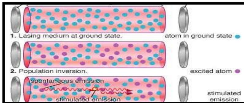
Figure (1.4): shows the emission process in the laser [5].
