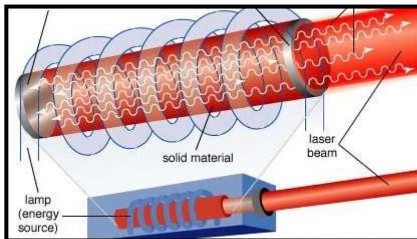
Figure (1.3): Shows the laser pumping process [5].
