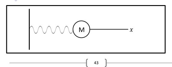
This force will be countered by other forces called restor fource, equal to the amount and in contrast to the direction, so that the movement can be described according to Newton's equation and Hawke's law.
