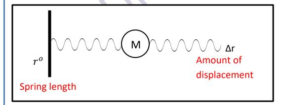
This system consists of a mass (m) attracted to the center by mechanical pull force (if the spring is frictionless) and the force of attraction (R) is known as restor force resulting from
