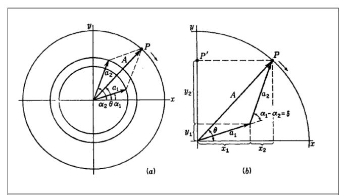
Fig. 1 Graphical composition of two waves of the same frequency, but different amplitude and phase.
