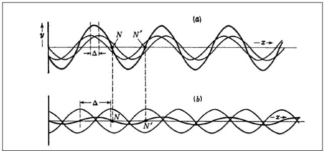
Fig. 3 Superposition of two wave trains (a) almost in phase and (b) almost 180' out of phase.
