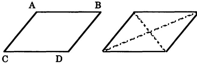
AB is parallel to CD. AC is parallel to BD. Both pairs of opposite sides are the same length. Both pairs of opposite angles are the same size. If diagonal lines (shown dashed above) are drawn to either pair of opposite angles the resulting triangles are congruent.
