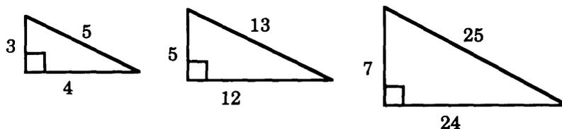
Note that any multiple of the ratios of these triangles is also a triplet, such as, 6:8:10, 10:24:26, etc.
