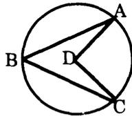
Angle ABC is an inscribed angle with endpoints on arc AC. Angle ADC is a central angle with endpoints on arc AC. Because they are formed by the same arc, angle ABC is one-half the measure of angle ADC.
