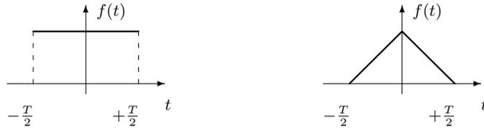
**Fig. 1.4.** "Constant" (left); "Triangular function" (right). We only show the basic intervals for both functions
