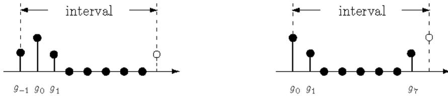
**Fig. 4.7.** Resolution function  $\{g_k\}$ : without wrap-around (*left*); with wrap-around (*right*)
