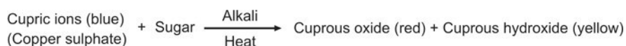
Fig. 1.9: Principle of Benedict's qualitative test for sugar in urine. Sensitivity is 200 mg of glucose/dl
