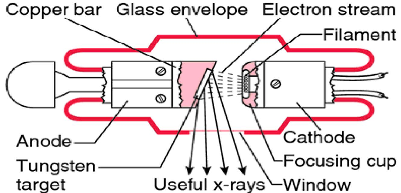
**Figure Construction of stationary Anode x-ray**
