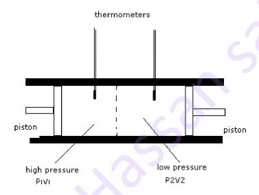
This effect was first observed in an experiment conducted by James Joule and Thomson in 1852 in which they flowed high pressure air through a small porous plug causing the pressure to drop. Joule and Thomson noted that the air was cooled by this procedure (which is a good approximation of an isenthalpic process (process done at constant enthalpy)).
