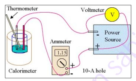
Q) Calculate the calorimeter constant, If pass a current of 10.0 A from a 12 V supply for 300 s, and the observed rise in temperature is 5.5 K.
