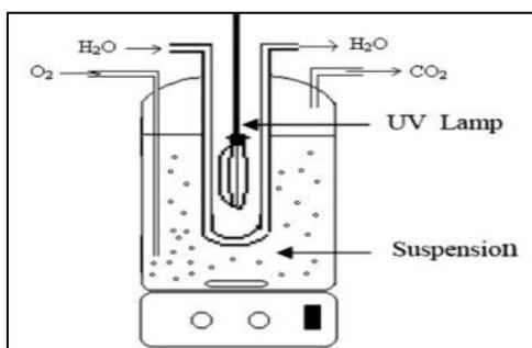
Photocatalytic experiments were performed in batch cylindrical photoreactor with a capacity of 2 L (Fig. 2). The reactor was made from quartz glass, which made possible the transfer of the irradiation. The reactor was exposed to a luminous source composed of a high-pressure mercury lamp (Philips HPK 125 W), placed in axial position inside a cooling water jacket system positioned inside the inner part of the reactor, containing the aqueous solution of phthalic acid. The agitation was assured by
