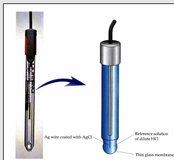
Fig. (3-17) : A glass electrode consists of a silver wire coated with silver chloride that dips into a reference solution of dilute hydrochloric acid. The hydrochloric is separated from the test solution of unknown pH by a thin glass membrane. When a glass electrode is immersed in the test solution, its electrical potential depends linearly on the difference in the pH of the solutions on the two sides of the membrane.
