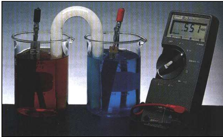
Fig. (2-19) : The cell potential is measured with an electronic voltmeter, a device that draws negligible current so that the composition of the cell does not change during the measurement. The display shows a positive value when the (+) terminal of the meter is connected to the cathode of the galvanic cell.
