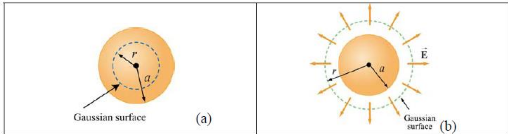
Figure 4.2.15 Gaussian surface for uniformly charged solid sphere, for (a) r \leq a , and (b) r > a .
