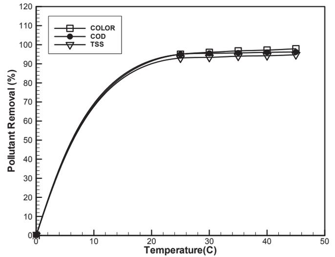
**Fig. 6.** Effect of temperature on the removal efficiencies of COD, TSS and color ( $CD = 4 \text{ mA/cm}^2$ ,  $RT = 10 \text{ min}$ , rotational speed = 150 rpm,  $\text{pH} = 4.55$ ).
