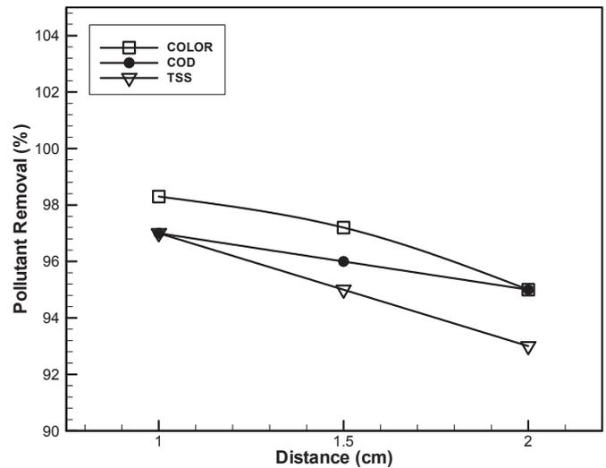
**Fig. 7.** Effect of inter electrode distance on removal efficiency of COD, TSS and color ( $CD = 4 \text{ mA/cm}^2$ ,  $RT = 10 \text{ min}$ , rotational speed = 150 rpm,  $\text{pH} = 4.55$  and  $T = 25 \text{ }^\circ\text{C}$ ).
