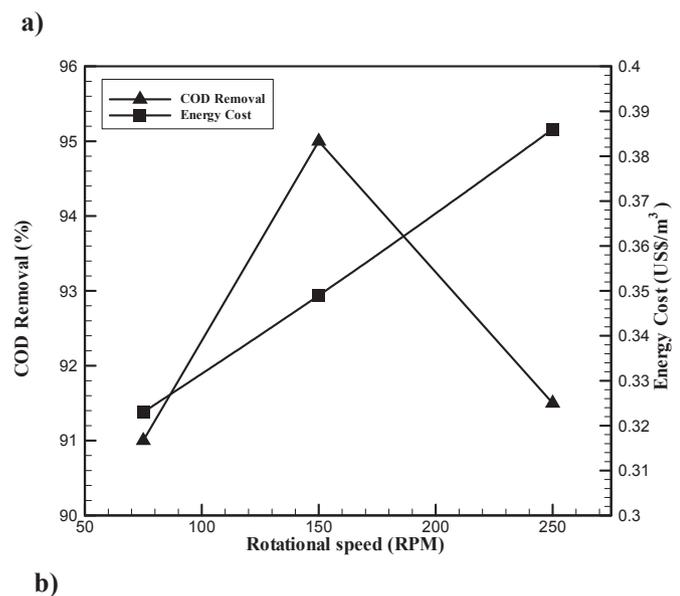
Fig. 3. a) Effect of current density and rotational speed on electrical energy consumption at reaction time = 10 min; b) Effect of rotational speed on COD removal and energy cost at CD = 4 mA/cm² and reaction time = 10 min.
