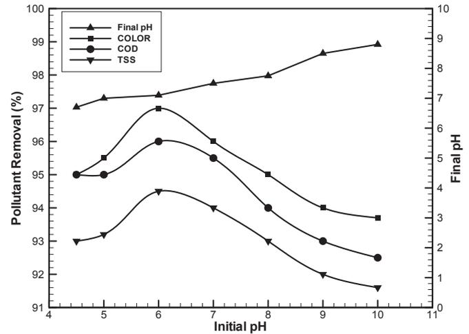
Fig. 4. Influence of initial pH on COD removal under optimal conditions (CD = 4 mA/cm², RT = 10 min, rotational speed = 150 rpm).
