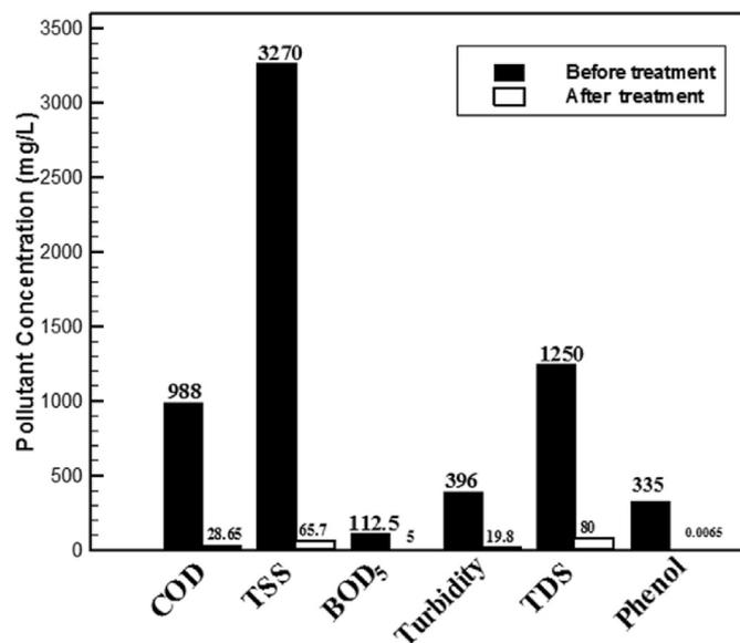
Fig. 8. The removal efficiency of various variables of the textile wastewater under optimal condition (CD = 4 mA/cm<sup>2</sup>, RT = 10 min, rotational speed = 150 rpm, pH = 4.57, Temperature = 25 °C, IED = 1).
